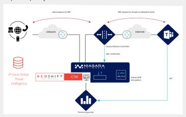
Niagara's Advanced Packet Brokers - enhanced with the award-winning Open Visibility Platform (OVP) and the pluggable Packetron acceleration module—solve this challenge by extending packet broker functionality with third-party virtual hosting and advanced packet processing. This enables robust TLS decryption, deep packet inspection, and full network intelligence (L2–L7), allowing organizations to maintain high-quality UC services while protecting against threats and ensuring compliance.
