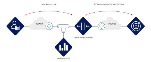
End user clients, either remote or connecting through an enterprise network connect to a Session Border Controller (SBC) which hides the network topology and protects the service provider or enterprise packet network.
