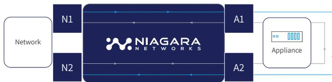
Figure 3: Inline deployment
